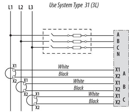
*Diagram 5: 3-Phase 4-Wire Wye Direct Voltage Input*
