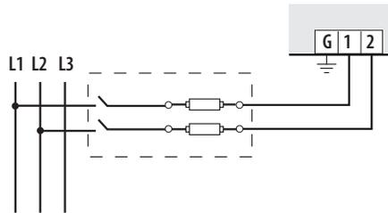
*Line to Line from 90 VAC to 600 VAC (UL). In UL installations the lines may be floating (such as a delta). If any lines are tied to an earth (such as a corner grounded delta), see the Line to Neutral installation limits. In CE compliant installations, the lines must be neutral (earth) referenced at less than 300 VAC<sub>L-N</sub>*
