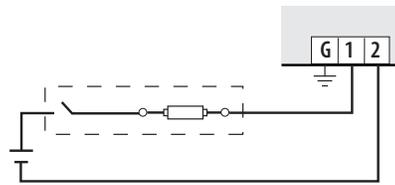
*DC Control Power from 125 VDC to 300 VDC
