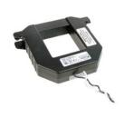
H681x-xxx 5 Amp split-core current transformers (CTs) provide secondary amperage proportional to the primary (sensed) current. For use with power meters, data loggers, chart recorders, and other instruments, the H681x Series 5 Amp CTs provide a cost-effective means to transform electrical service amperages to a 0 to 5 Amp level compatible with monitoring equipment.
