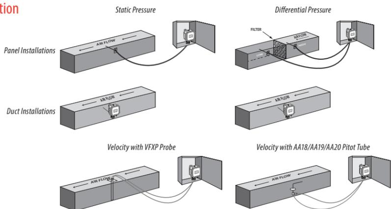
For velocity applications, use the VFXP Series air velocity/measurement probe or AA18, AA19 or AA20 velocity pitot tubes. For use with the PX3P (panel) and PX3U (universal) models in Velocity mode only. Sold separately.
