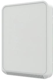
The CWE2 and CWV2 Series of air quality sensors for living space are for use with BAS controllers designed to accept 4 to 20mA, 0 to 5 Vdc or 0 to 10 Vdc outputs. These sensors measure CO<sub>2</sub> levels using a dual-beam, non-dispersive infrared (NDIR) technology.
