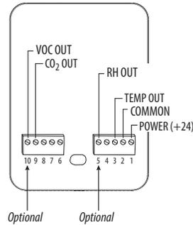
**CW2L/CW2T DISPLAY MODELS WITH RTD/THERMISTOR**
