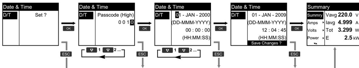
1. Press **OK** when you are prompted to set the date and time when the meter is powered up.
