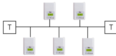
Figure 3.2 Doubly Terminated Bus Topology
