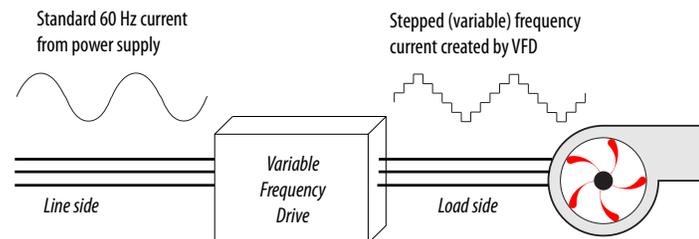
An embedded microprocessor controls the overall function of the VFD, while user programming governs the parameters the VFD uses to control the motor on the load side.
