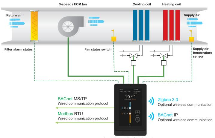
Low-Voltage Fan Coil Controller
