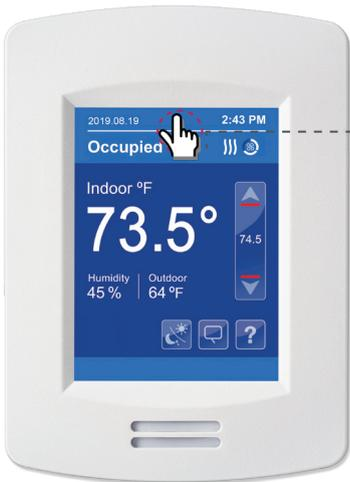
Touch and hold this point for 3 seconds to enter set-up mode
