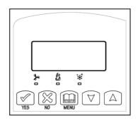
It is possible to bring up the user menu at any time by depressing the MENU key. The status display automatically resumes after exiting the user-configuring menu.
