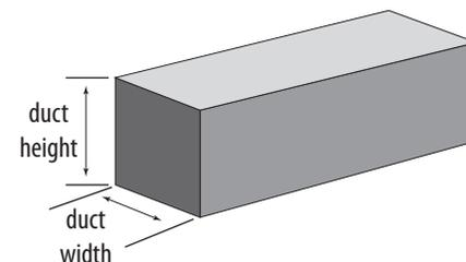
For rectangular ducts, calculate area using the formula
