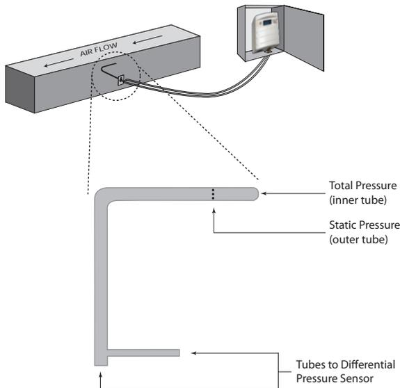
The sensor's output will be the velocity pressure (the difference between total pressure and static pressure in the duct).
