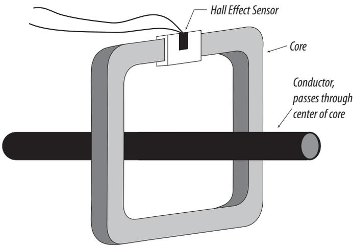
The drawback for Hall Effect technology occurs when the core is subjected to a strong current spike, power surge, or external magnetic field. These forces cause the core's magnetic field to be permanently altered, such that the pre-programmed zero level is no longer accurate. Subsequent outputs from the sensor will be skewed. It is possible to recalibrate a damaged sensor, but this involves labor and costly downtime.
