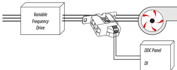
When first installed, the H614 learns the system amperage curve by storing the sensed values for normal operation at twenty frequency bands over the entire frequency range. During normal operation, the H614 monitors for changes in current greater than  $\pm 20\%$  of the learned load at each frequency band. This allows the sensor to distinguish between a reduced amp draw due to normal changes in the system and an abnormal amperage drop due to belt loss or other mechanical failure.
