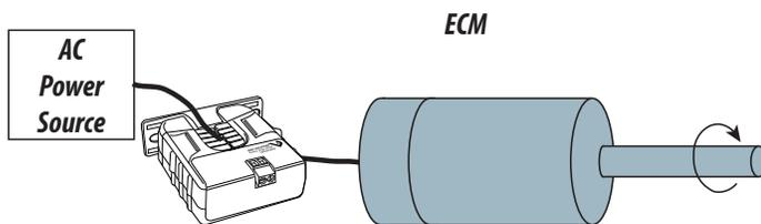
Monitoring can be accomplished in two ways, either using a current sensor with analog output or using a current switch.
