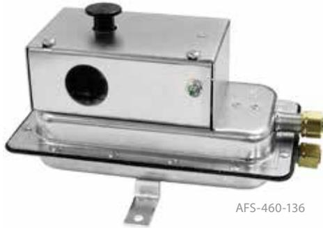
The AFS-460 is a general purpose airflow proving switch designed for 120 Vac (AFS-460-136) or 24 Vac (AFS-460-137) HVAC and Energy Management applications where a manual reset switch with DPDT contacts is desirable. It may be used to sense positive, negative, or differential air pressure.
