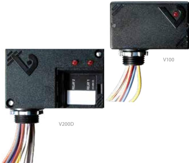
Victory 100 and 200 Series 10 A enclosed relays are pilot-duty relays in an easy-to-use nipple mount enclosure. The V100/V200 Series provide quick relay mounting without a dedicated field enclosure, making them ideal for retrofit projects. Field-selectable high and low voltage coil inputs provide on-site versatility.
