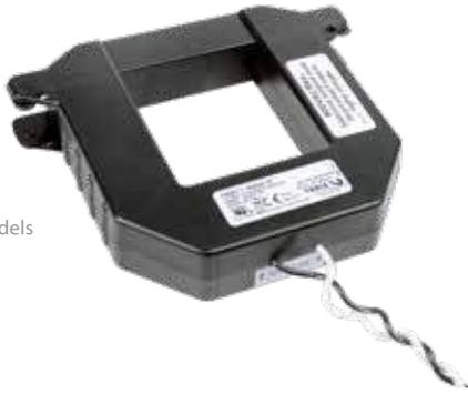
The H681x Series of 1 volt and 0.333 volt split-core current transformers (CTs) provide secondary AC voltage proportional to the primary (sensed) current. For use with power meters, data loggers, chart recorders, and other instruments, the H681x-V series CTs provide a cost-effective means to transform electrical service amperages to a voltage compatible with monitoring equipment.
