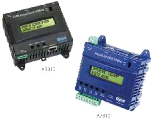
The A7810 AcquiLite™ and A8810 AcquiSuite™ data acquisition server for embedded applications allows users to collect energy data from meters and environmental sensors and send it via Modbus communication protocol (wired or wireless using the H8830) to IP-based applications. No software is required. Operation is plug-and-play, and information can be accessed using any web browser. The A7810 supports four pulse inputs, while the A8810 supports Modbus serial input.
