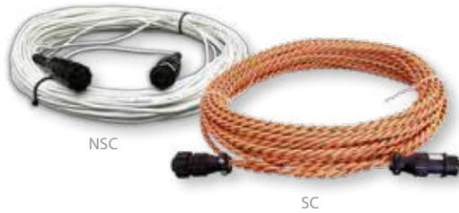
Sensing and non-sensing cables are designed for use with Zone and Distance Read panels. The sensing cables detect the presence of detectable liquid, and send a signal to the panel. The panel generates an alarm and pinpoints the location of the leak or spill along the cable's length. Sensing cables are designed for high accuracy and maximum reliability.
