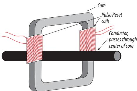
The Pulse Reset coils surround the metal core. As the core's magnetic field fluctuates, the coils periodically demagnetize the core. If a power surge occurs, this frequent neutralization of the magnetic field prevents any lasting effect on the core.
