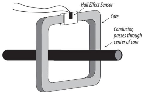
The drawback for Hall Effect technology occurs when the core is subjected to a strong current spike, power surge, or external magnetic field. These forces cause the core's magnetic field to be permanently altered, such that the pre-programmed zero level is no longer accurate. Subsequent outputs from the sensor are skewed. It is possible to recalibrate a damaged sensor, but this involves labor and costly downtime.
