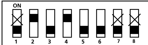
Standard N2 Configuration: X=unused. 2-wire 9600 Baud No Parity (Default Only)
