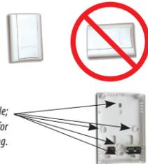
Five screwholes available; use a minimum of two for secure mounting.
