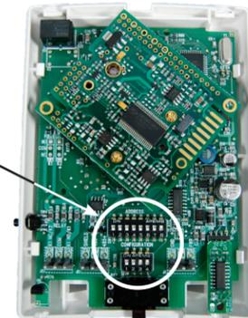
DIP switches, located on backside of board, Top row: Address switches Bottom row: Configuration switches
