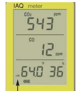
Wet Bulb Temperature Indicated by "WB" in the display
